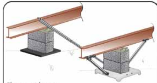
Shown with two longitudinal struts for Wind Zones II & III
