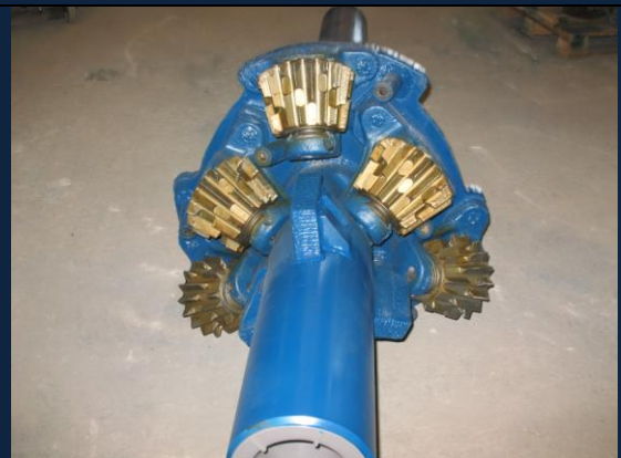
New 36" 6 pt. Custom Hole Opener Body with Sealed Bearing Tooth Cutters
