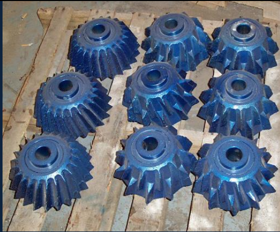
New sealed Bearing Tooth Cutters for BRI Custom Hole Opener Body
