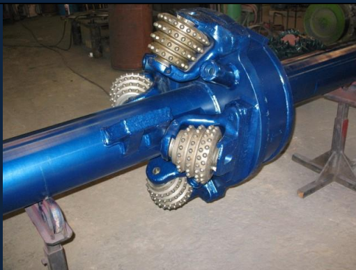
New 36" 4 pt. Custom Hole Opener Body with Sealed Bearing TCI Cutters
