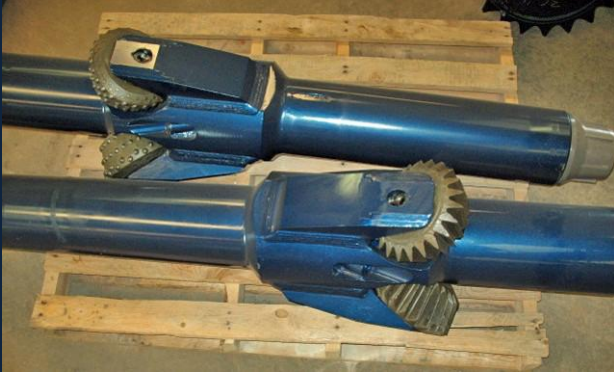
New BRI Security Type Hole Opener Bodies with replaceable Tooth or TCI Cutters
