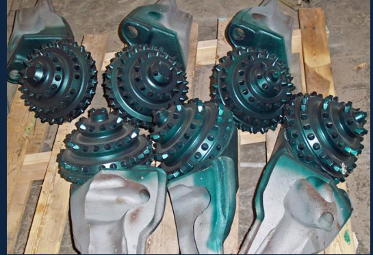
New Sealed Bearing TCI segments for BRI Split Type Hole Openers
