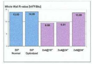
conditions. Unlike stick and batt construction, which can be subject to poorly installed - even missing - insulation, the nature of SIPs is such that the structural and insulative elements are joined as one. There are no hidden gaps, because a solid layer of foam insulation is integral to panel construction.
